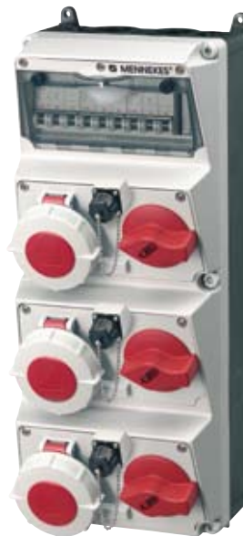
☼☼ IP 67 AMAXX® receptacle combination for containers and terminals, pre-wired for installation, enclosure size: 520 x 225 mm, black base, front cover electric grey RAL 7035, hinged to the side, fusing under transparent cover 3 CEE 32A, 4p, 400V, 3h switched, with mechanical DUO interlock 3 MCB's 32A, 3p, C 3 monitoring sockets MS3102E 14S2S Connection:
