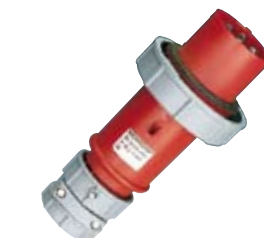
☼☼ IP 67 CEE plug PowerTOP with cable gland and external cable grip. Contact pins sealed with gaskets.
